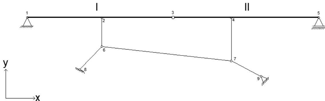
a) ZGLOBNI ŠTAPOVI SPOJENI S TIJELIMA SU PARALELNI SA SILOM U POMIČNOM ZGLOBU
