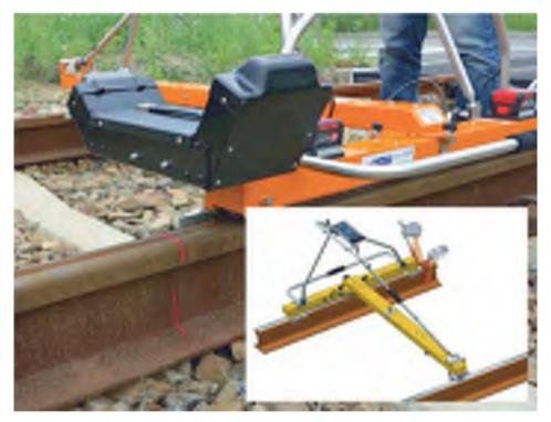
Figure 2 Track geometry and rail head profile trolley
