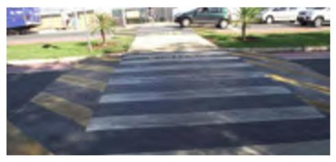
Figure 4 Example of elevated curbside to facilitate boarding of wheelchair users
