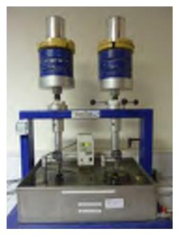
Figure 1 Machine to measure the indentation according to the standards EN 12697-20 and EN 12697-21
