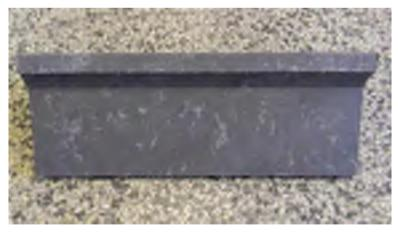
Figure 4 Plastic sleeper anchor after abrasion resistance test
