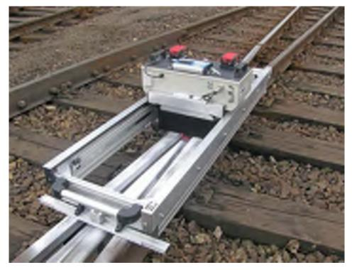
Figure 6 Optical system for track and turnout measurement
