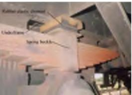
Figure 5 The rubber-metal elastic element instaled in suspension
