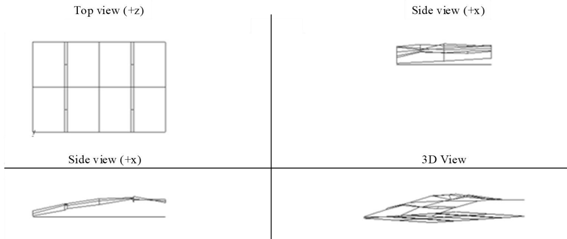
Figure A.IV.1. Experimentally determined mode shapes ( \phi_t^{exp} ) of the span slab of pedestrian suspension bridge over Drava River for corresponding natural frequency ( f_t^{exp} ) ( t = 1, \dots, 10 )
