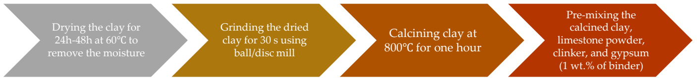
Figure 3.2 Steps involved in the preparation of LC3 in the lab for this study.
