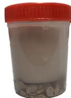
Figure 4.3 Samples curing in their own pore solution.
