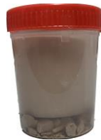
Figure 4.3 Samples curing in their own pore solution.
