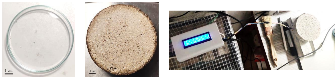
Figure 4.2. Water vapour permeability examination set: (a) makeshift test cups; (b) specimen prepared for testing; (c) thermohygrometer tracking T & RH conditions
