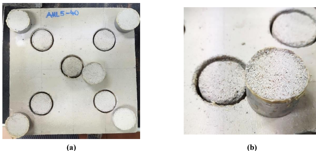
Figure 4.45. AHL 5-40-M mortar slab after pull-off test: (a) five test regions; (b) detail of failure mode (B)
