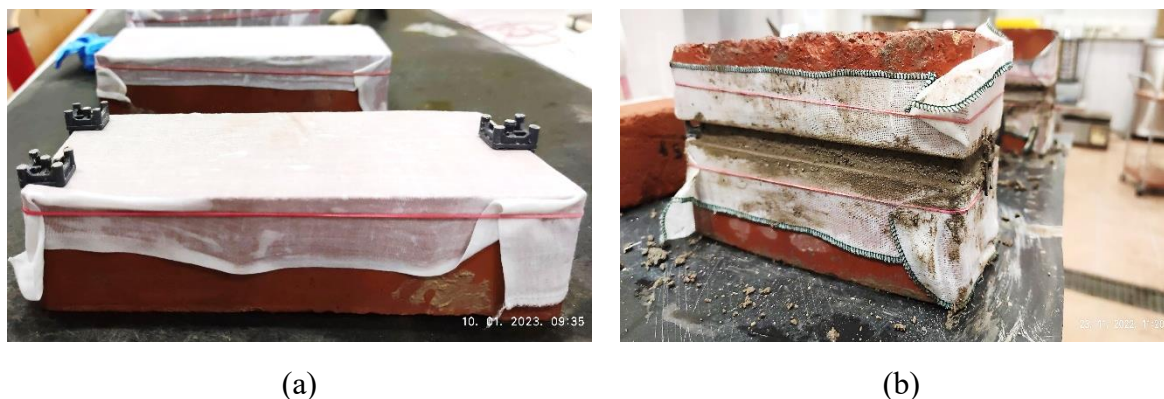
Figure 4.46. Preparation of mortar beds: (a) set of brick units; (b) mortar and brick coupled units
