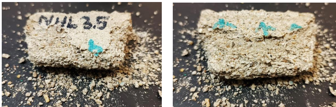
Figure 4.52. The NHL 3.5-M 'S2-b' specimen, displaying prominent degradation after enduring 11 cycles
