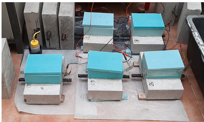
Fig. 2. The setup for the accelerated corrosion process.
