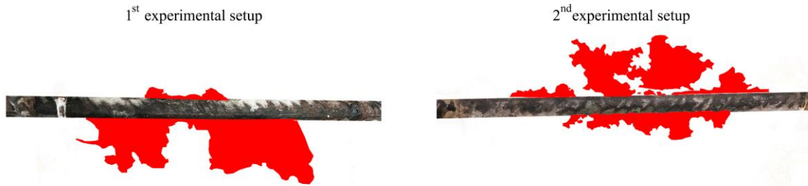
Figure 4. Comparison of the corrosion pattern in two experimental setups (originally presented in Paper II).
