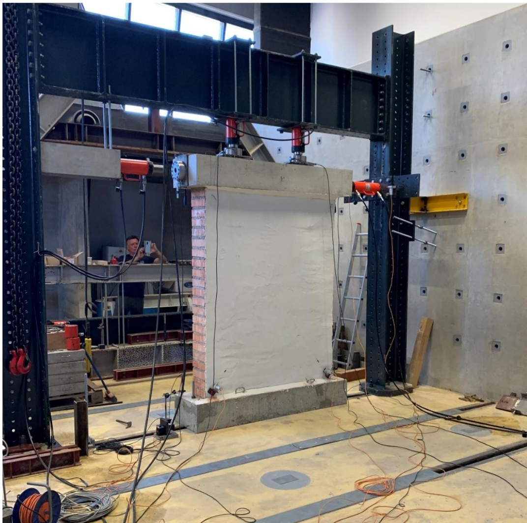
Figure 4.38 Testing of a FRCM pier
