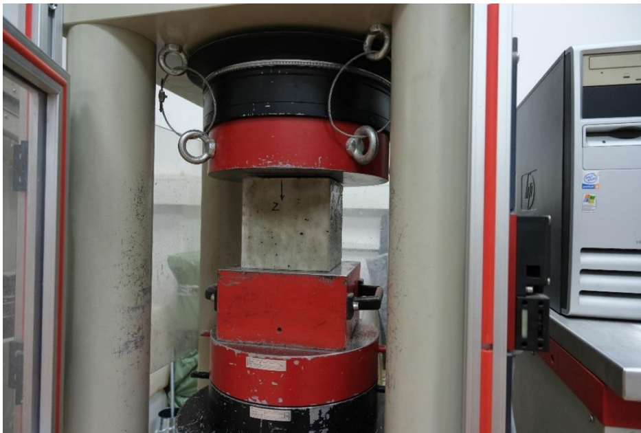
Figure 4.8 Compression strength testing of concrete cubes
