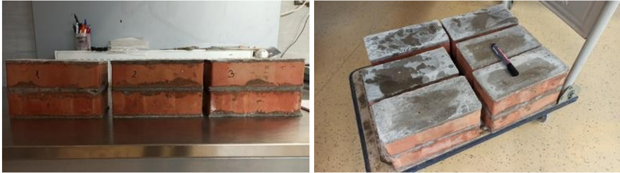
Figure 4.9 Test specimens for the determination of the compressive strength of masonry units
