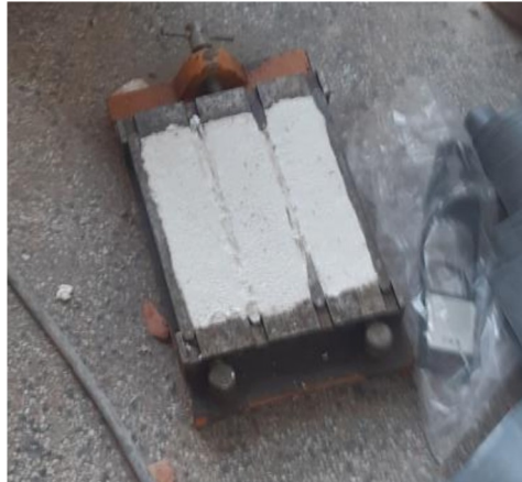
Figure 4.11 Three samples for the compressive strength test of hardened mortar
