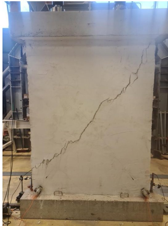
Figure 4.49 Final failure mechanism of FRCM 3 pier
