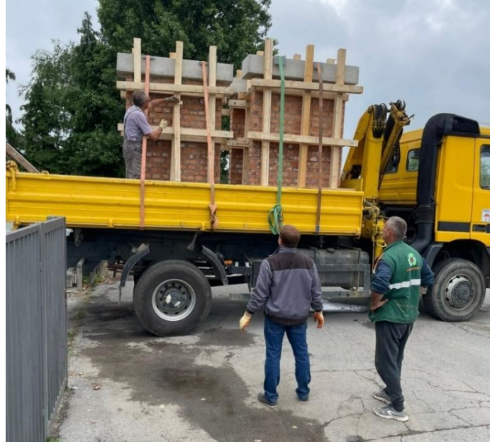
Figure 4.16 Transportation of masonry piers to the laboratory
