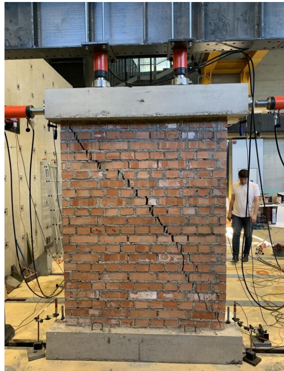
Figure 4.46 Final failure mechanism of FRCM 2 pier
