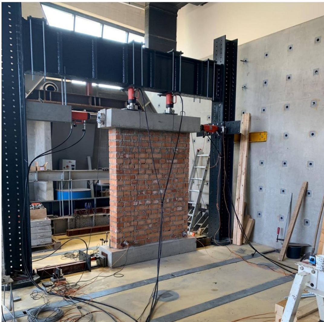
Figure 4.21 Testing of an URM pier
