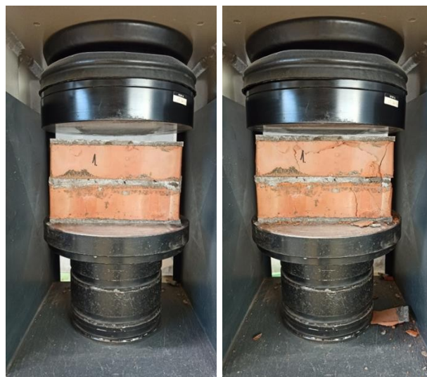
Figure 4.10 Test specimens before and after the testing
