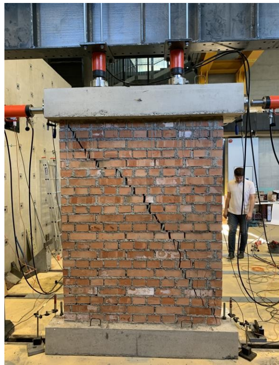
Figure 4.46 Final failure mechanism of FRCM 2 pier
