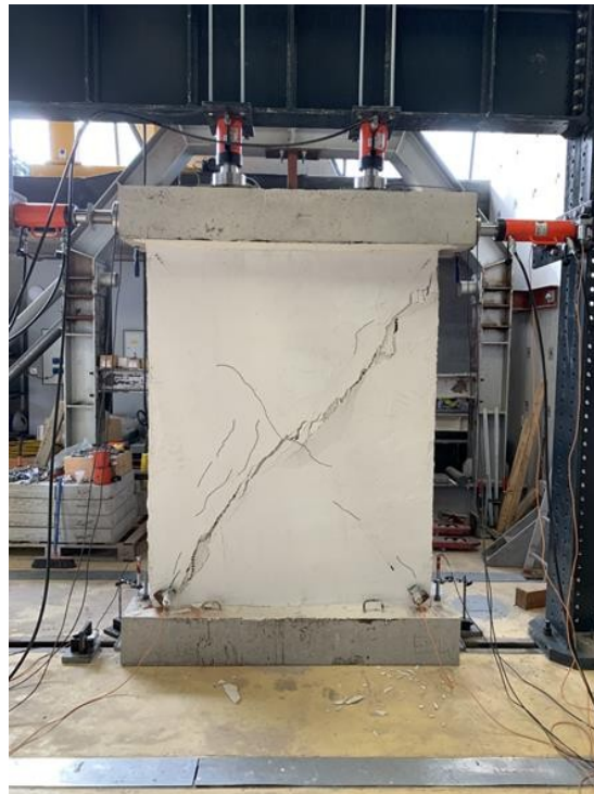
Figure 4.59 Final failure mechanism of CFRCM 2 pier
