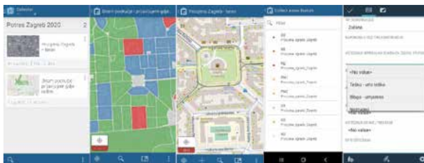
Figure 11. Filling-in the inspection form using Collector for ArcGIS
