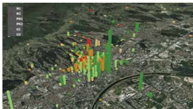
Figure 31. Damage to cultural heritage buildings according to usability tags (colours) and gross floor area (columns) on 3D aerial view of the City of Zagreb
