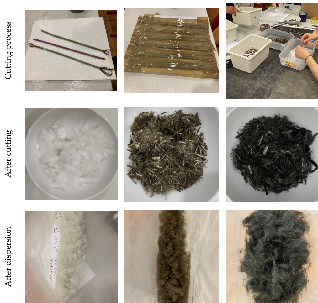
Figure 1. Visual appearance of the waste fibres used, from left to right: AR-glass, basalt and carbon fibres.
