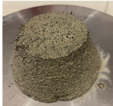
Figure 3. Improper dispersion of carbon fibres in fresh mortar.
