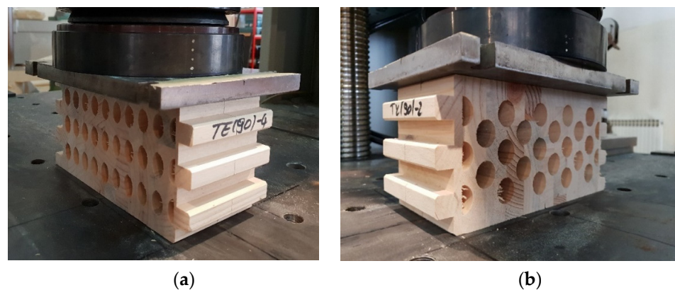
Figure 23. Timber samples during the experimental test of compression strength perpendicular to the grain in the direction of the stronger axis. (a) elliptical cavities; (b) circular cavities.
