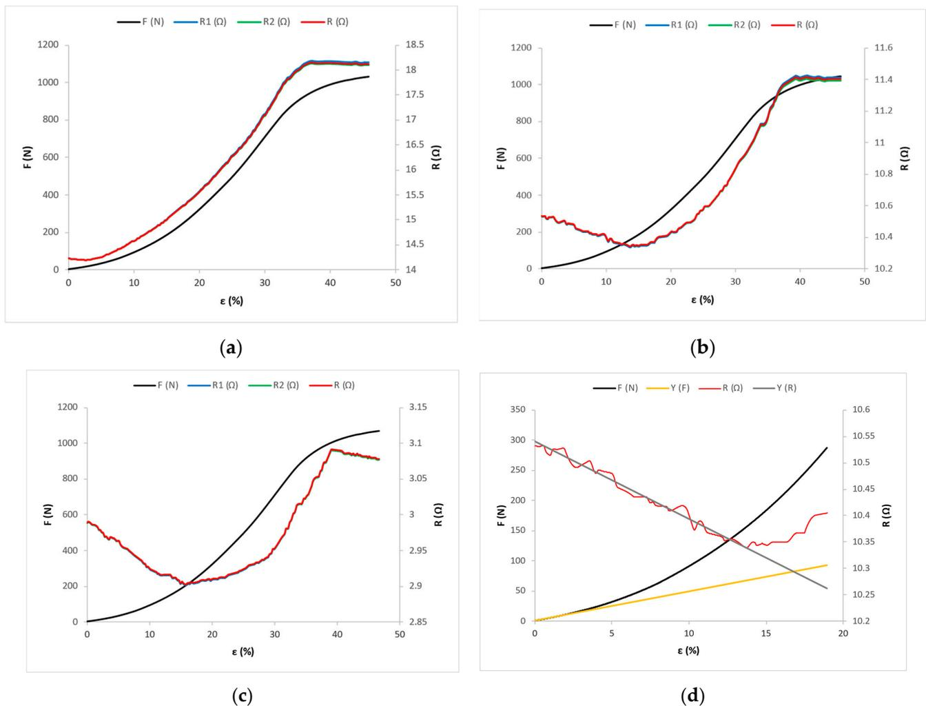
**Figure 6.** Force–elongation ( $F$ - $\epsilon$ ) and electrical resistance–elongation ( $R$ - $\epsilon$ ) diagrams for fabric samples cut in the warp direction: (a) for sample X-0; (b) for sample Y-0; and (c) for sample Z-0. (d) Experimental and mathematical models of  $F$ - $\epsilon$  and  $R$ - $\epsilon$  curves for sample Y-0.
