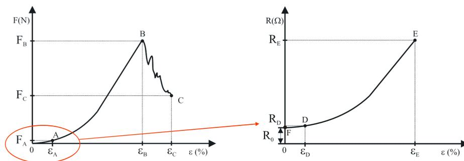
Figure 2. Characteristic diagrams of the tensile force–elongation ( $F$ - $\epsilon$ ) curve of the woven fabric and the electrical resistance–elongation ( $R$ - $\epsilon$ ) curve of the conductive fabric yarn.
