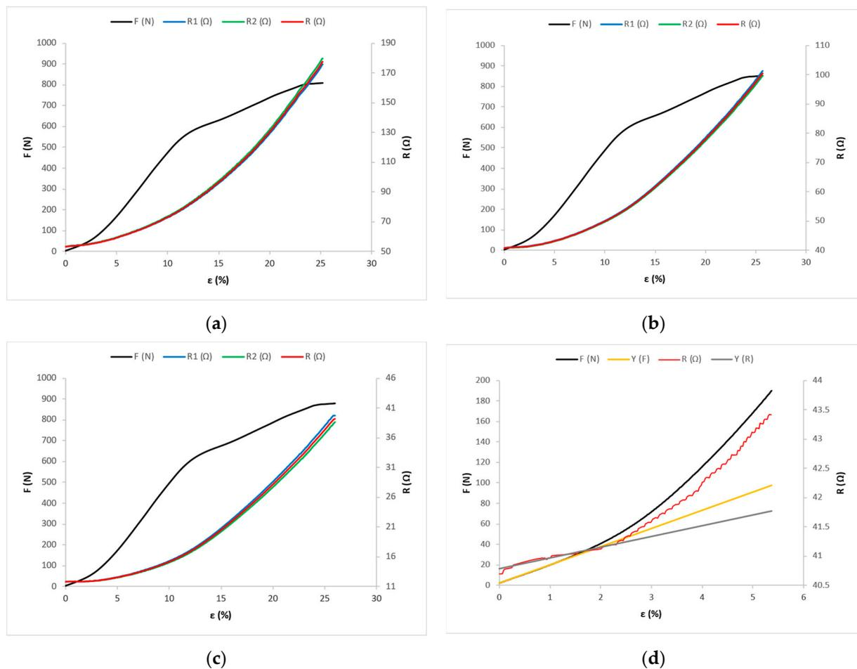
**Figure 8.** Force–elongation ( $F$ - $\epsilon$ ) and electrical resistance–elongation ( $R$ - $\epsilon$ ) diagrams for fabric samples cut in the weft direction: (a) for sample X-90; (b) for sample Y-90; and (c) for sample Z-90. (d) Experimental and mathematical models of  $F$ - $\epsilon$  and  $R$ - $\epsilon$  curves for sample Y-90.
