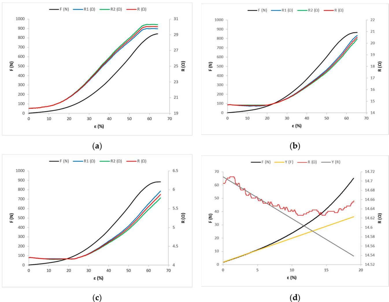
**Figure 7.** Force–elongation ( $F$ - $\epsilon$ ) and electrical resistance–elongation ( $R$ - $\epsilon$ ) diagrams for fabric samples cut at a 45° angle: (a) for sample X-45; (b) for sample Y-45; and (c) for sample Z-45. (d) Experimental and mathematical models of  $F$ - $\epsilon$  and  $R$ - $\epsilon$  curves for sample Y-45.
