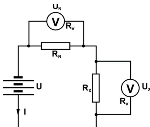
Figure 1. Scheme of the series measuring circuit.
