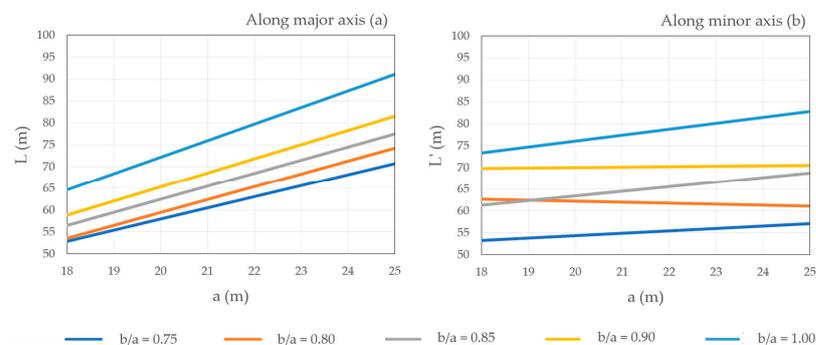
**Figure 9.** The linear dependency of the distance between the tangent of the entry radius and the tangent of the exit radius ( $L$  and  $L'$ ) and the major axis length ( $a$ ) for roundabout schemes with fixed ( $y$ ).
