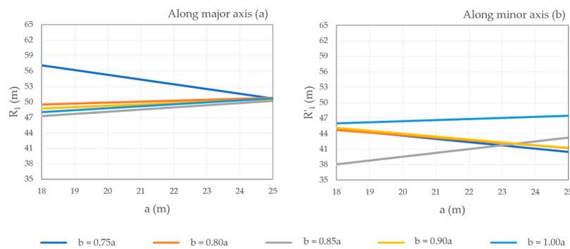
**Figure 11.** The linear dependency of the entry path radii ( $R_1$  and  $R'_1$ ) and the major axis length ( $a$ ) for roundabout schemes with fixed ( $y$ ).
