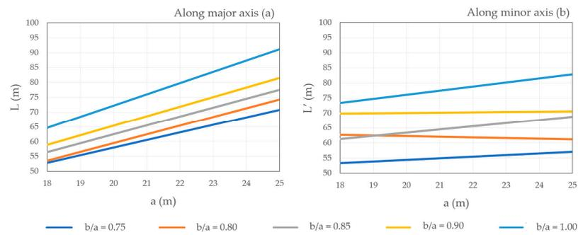
**Figure 4.** The linear dependency of the distance between the tangent of the entry radius and the tangent of the exit radius ( $L$  and  $L'$ ) and the major axis length ( $a$ ) for roundabout schemes with variable ( $y$ ).
