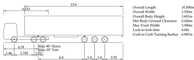
**Figure 2.** Design vehicle (Scania R500 LA6x2/4MNA tractor with a generic 13.6 m long and 2.55 m wide trailer).
