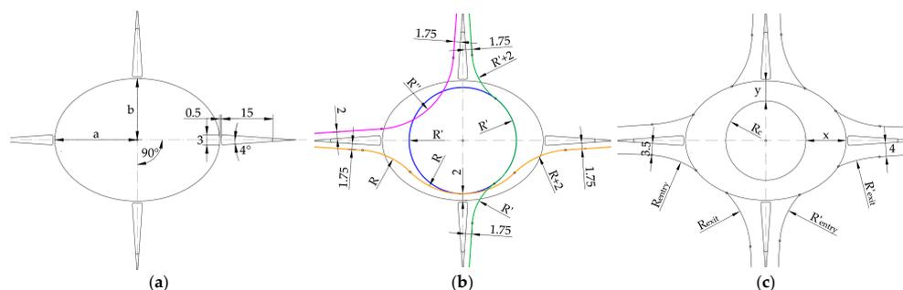
**Figure 1.** Roundabout design procedure. (a) Initial scheme; (b) Front axle center point path parameters and elements (path for the circular movement around the central island is shown in blue, path for the right turn is shown in pink, path for straight passage in major axis direction is shown in orange, path for straight passage in major axis direction is shown in green); (c) Final roundabout design elements.
