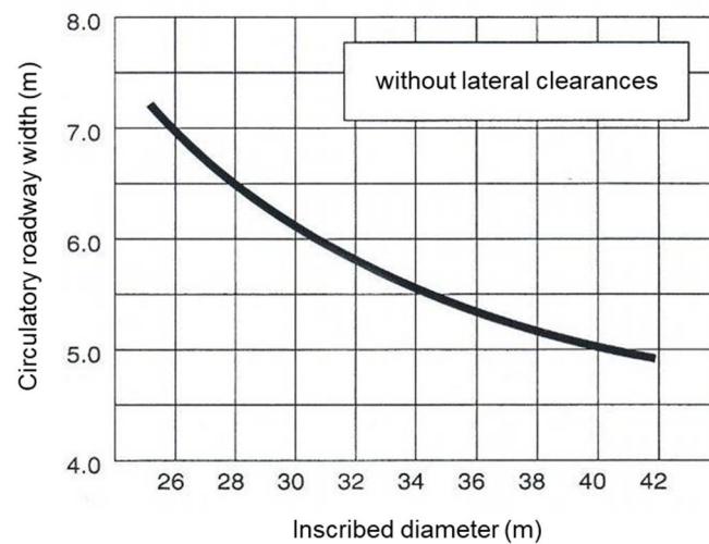
Figure 7. Minimum circulatory roadway width (together with apron width) depending on the roundabout inscribed diameter [12].
