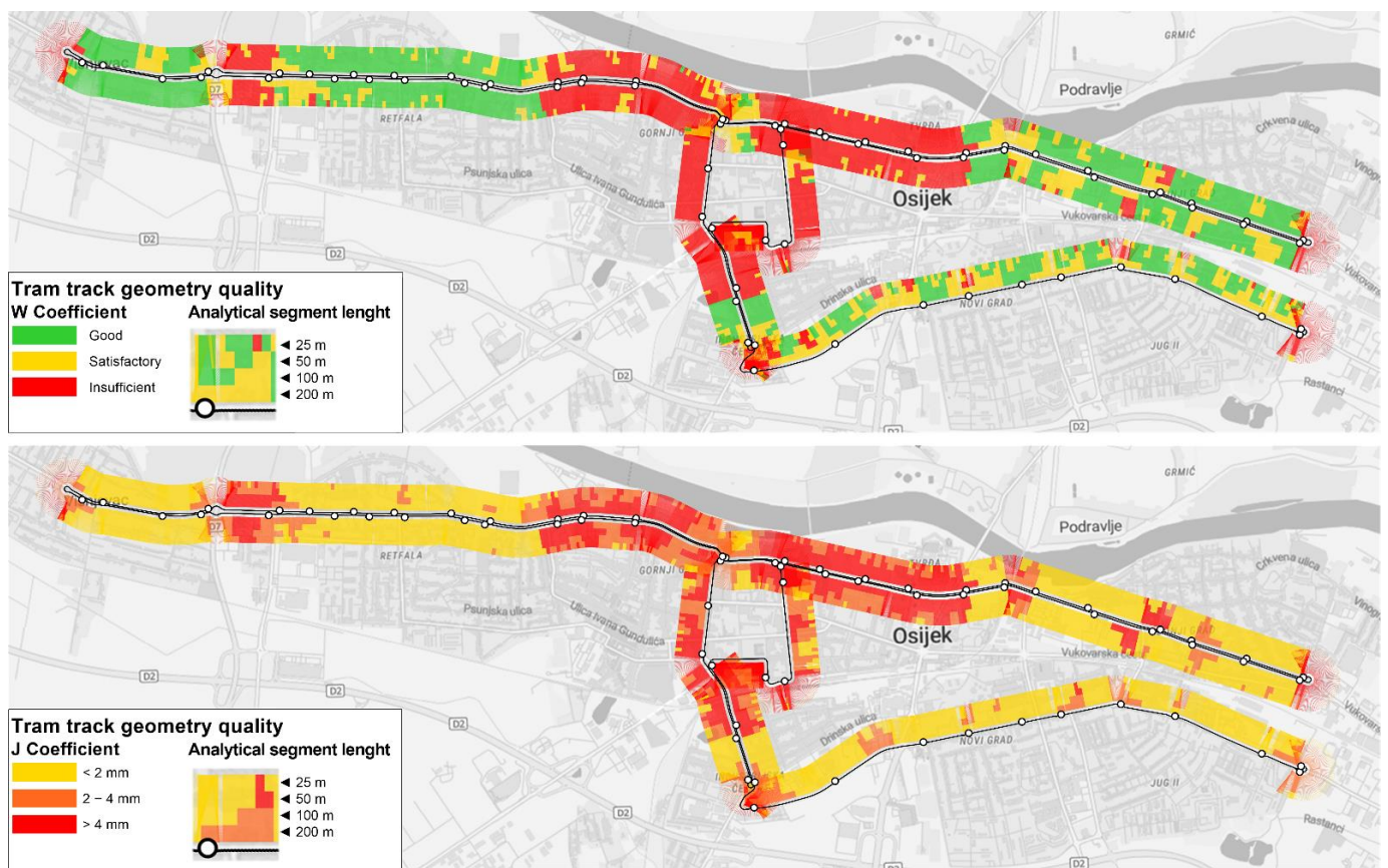
Figure 8. Track quality W and J index distribution along the tracks.
