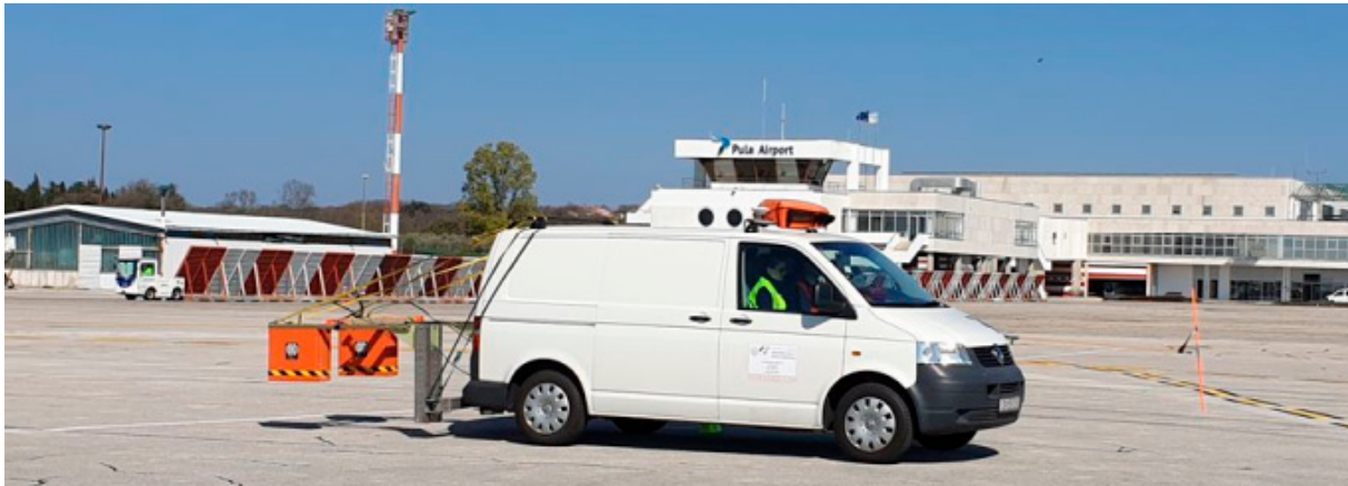
Figure 2. Measurement vehicle at the Pula Airport with Ground-penetrating radar (GPR) antennas.
