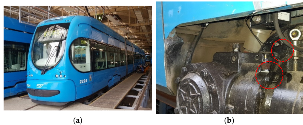
Figure 5. (a) Tram TMK2224 in the position for accelerometer mounting; (b) vertical and transverse accelerometers at the central bogie.
