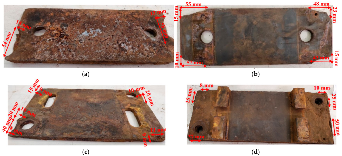
Figure 14. Condition of the steel plate after testing was completed: (a) ZG 3/2, (b) PPE, (c) DEPP, and (d) Zagreb 21-CTT.
