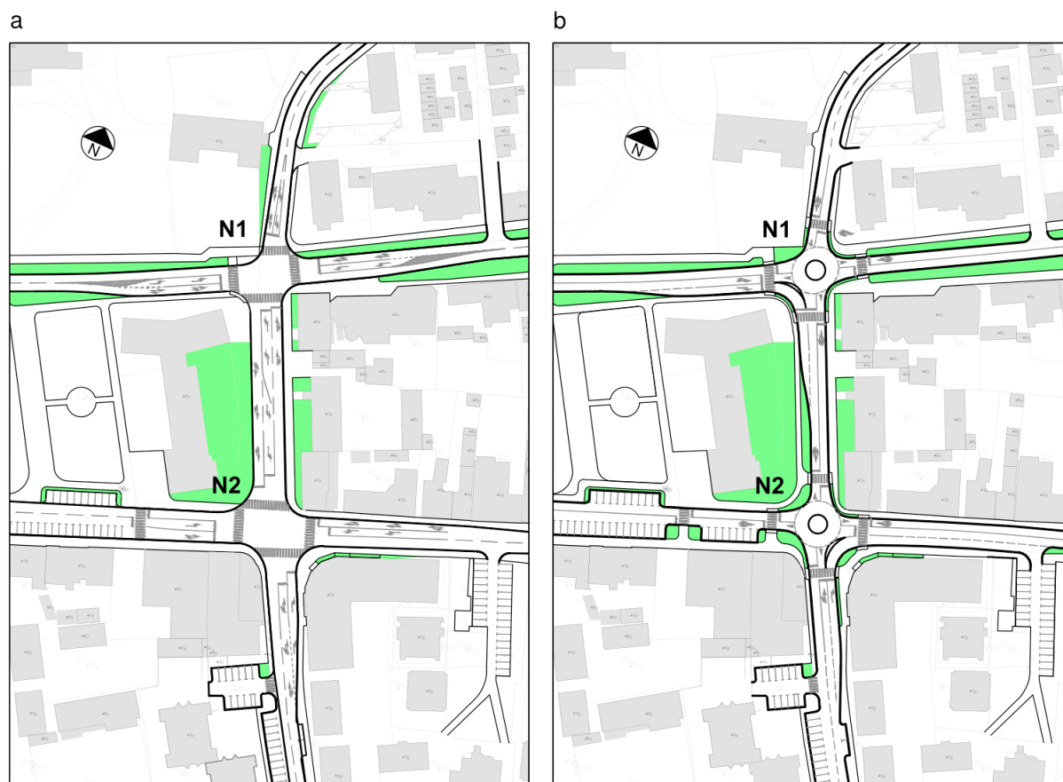
Fig. 3. Design of (a) current intersections; (b) planned intersections.
