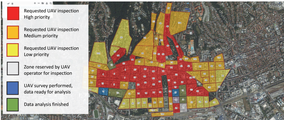
Figure 2. Zone definition and classification for UAV inspection
