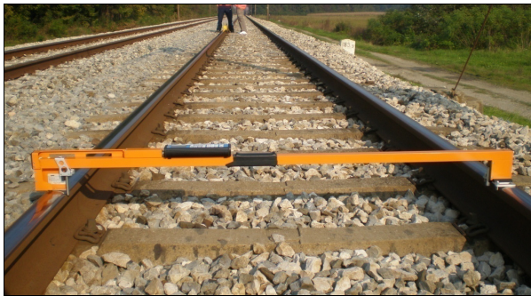
Figure 3 Manula track geometry measurement
