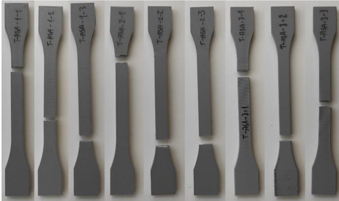
Figure 3.2 Nine 3D-printed specimens displaying various fracture zones (1, 2 and 3 represent the XY, XZ and ZX print direction, respectively)
