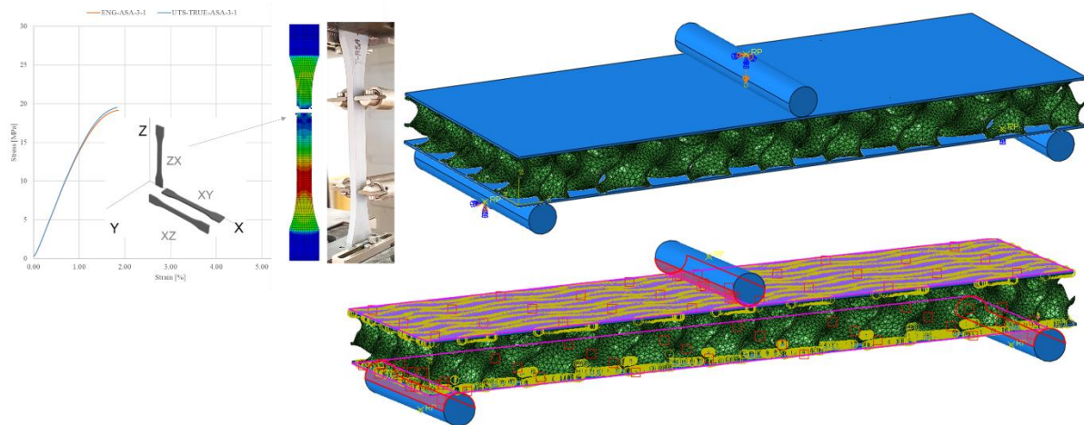
Figure 7.1 Material model set for FEM analysis of the sandwich panel with 3D printed core.
