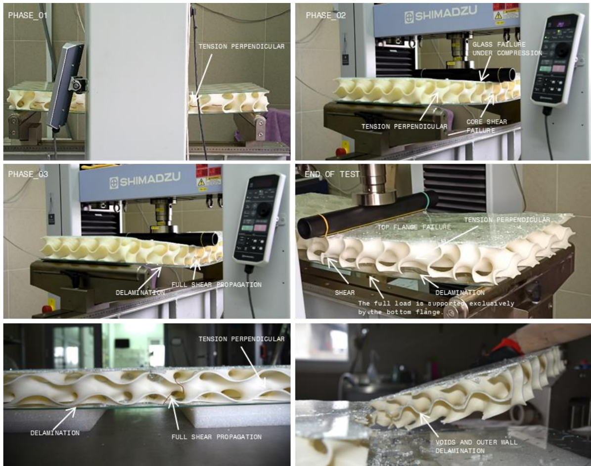
Figure 8.7 Snapshots from bending test by phases
