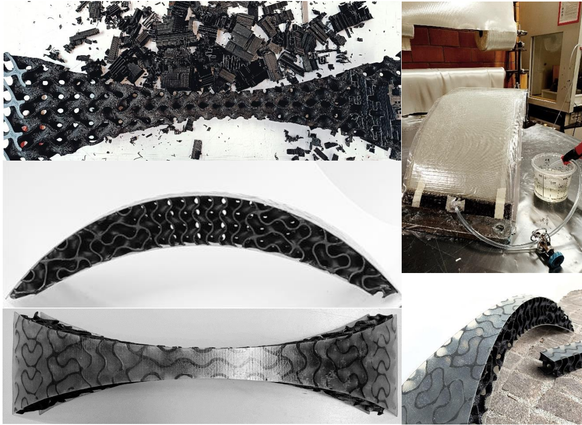
Figure 6.6 Production of the composite sandwich arch
