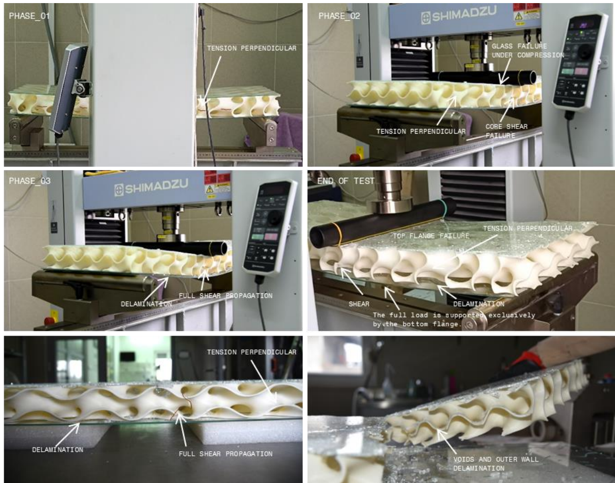
Figure 8.7 Snapshots from bending test by phases
