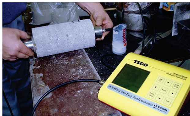
Figure 2 Measurement of ultrasound pulse velocity
