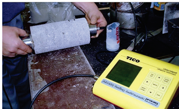
Figure 2 Measurement of ultrasound pulse velocity
