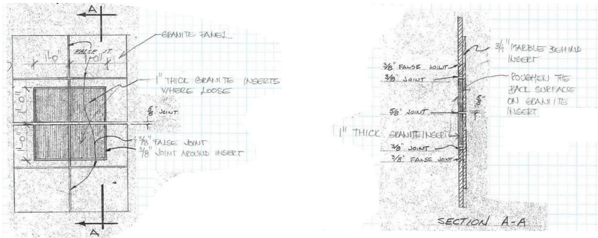
Figure 6 - Granite inserts attached with epoxy adhesive that has failed. As built conditions are different than designed
