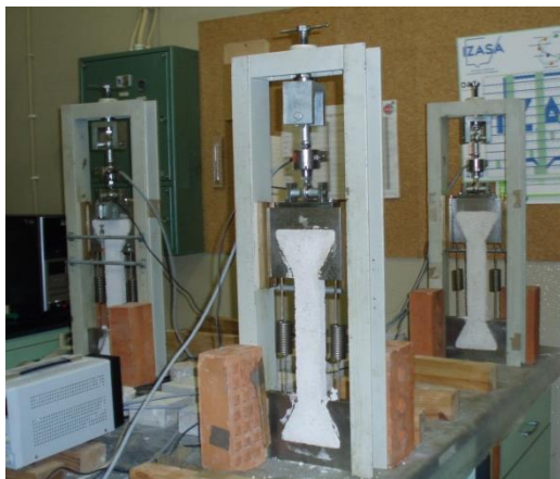
Figure 1 – Restrained shrinkage tests: a) Uniaxial test; b) Slab test
