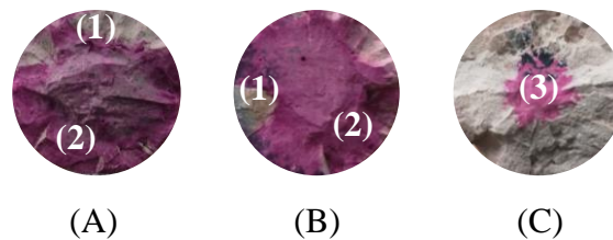
Figure 3: Carbonation depth measurement for 100PC (A), 60PC40S (B) and 30PC70S (C) sealed for 28 days and subjected to 28 days of accelerated \text{CO}_2 ingress. (1) Large carbonation depth due to superficial carbonation at the crack planes (2) Very limited carbonation in the sound (non-cracked) zones (3) uniform radial ingress
