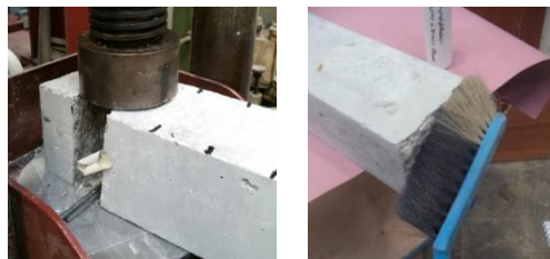
Figure 1: Cutting and Cleaning of concrete prisms
