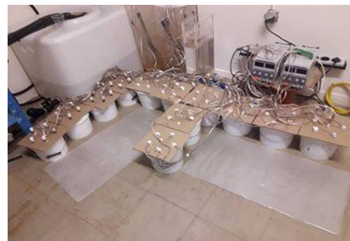
Figure 2: Procedure of accelerated electro-corrosion. (Left) Schematic representation, (Right) Experimental setup
