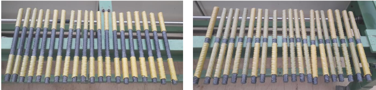
Figure 1: Preparation of the “long” specimens (exposed length 12cm – left) and “short” specimens (exposed length 2cm – right)
