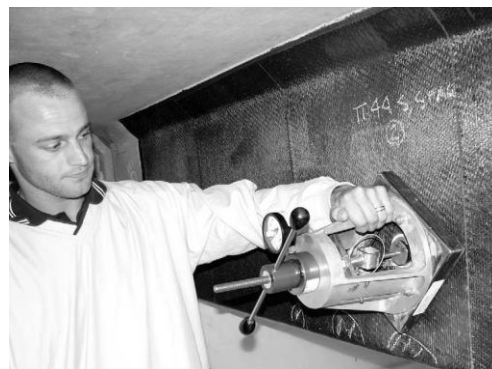
Figure 2: Tensile bond testing of the applied FRP
