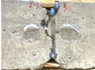
Figure 7: Release of repair agent outside the specimen
