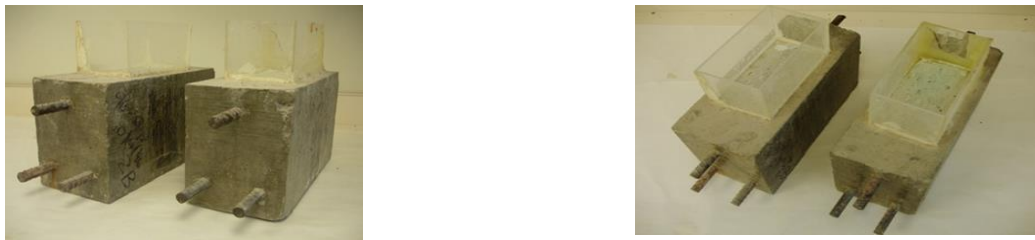
Figure 3. Example of ASTM G109 Test Blocks
