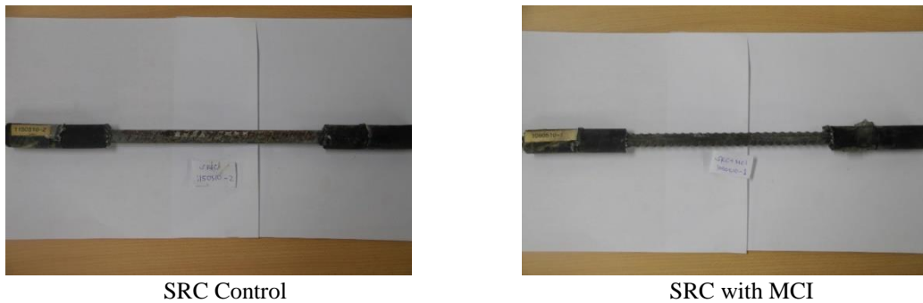
Figure 5 Reinforced steel removed from of SRC and SRC with MCI
