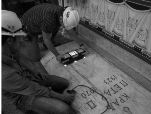
Figure 17: Determining the thickness of stone with GPR
