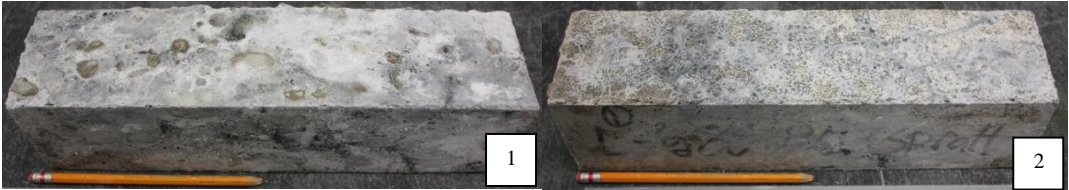
Figure 2. Visual Aspect of Slag-Based Concrete Prisms after 2 Years of Expansion Testing with NM Aggregates (1) and Sp Aggregates (2)
