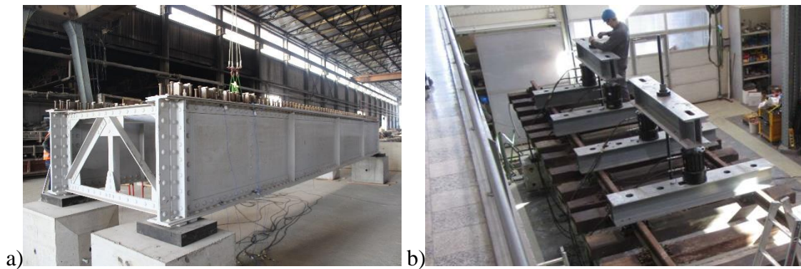
Figure 1: Bridge before deck casting with welded studs on the upper girder flange (a) and bridge with UHPFRC deck, sleepers and tracks mounted with sensors and testing equipment in the lab (b)
