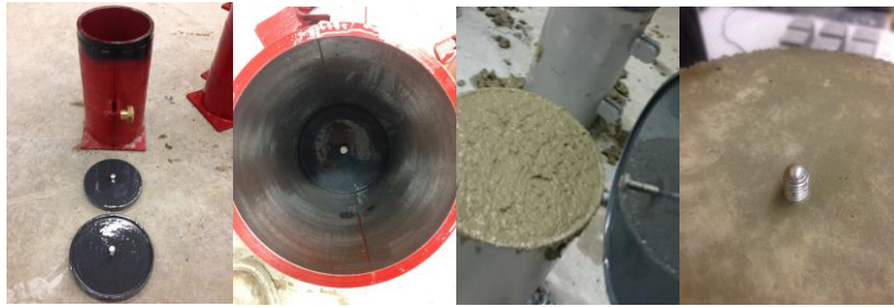
Figure 1: (a) Custom made mold with top and bottom plates holding embedded studs, (b) Concrete mold with bottom plate prior to casting, (c) Installing top plate with gauge pin, (d) embedded gauge pin following curing
