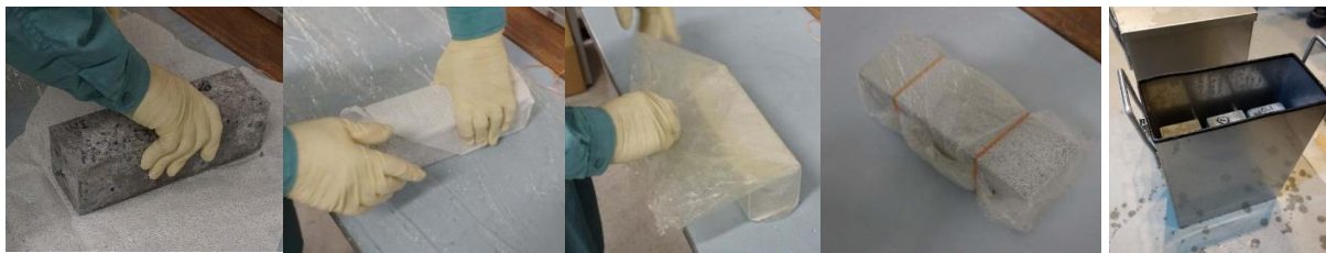
Figure 2: Examples of alkali-wrapping of concrete prisms.
