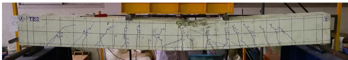
Figure 3: Failure of NSM FRP-strengthened beam TB2
