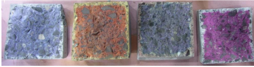
Figure 3: Colour change on a concrete sample determined with different indicators (from left to right: 0.1 % thymolphthalein, 0.5% curcumin, Rainbow Indicator, 1% phenolphthalein)
