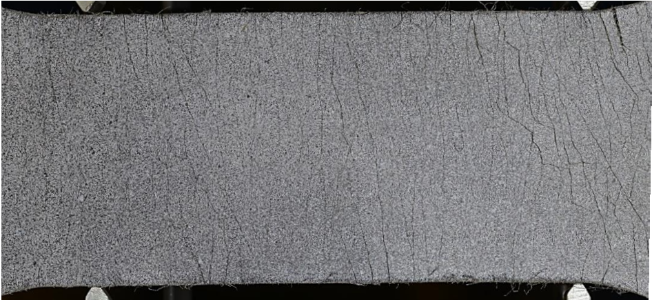
Figure 2: Close-up of the cracked surface of the ECC dogbone specimen after tensile testing. The longitudinal distance between pins is 110 mm and the transverse is 50 mm.
