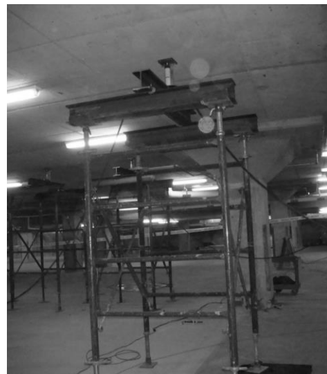
Figure 6: Load test set-up and load-deflection results after completion of slab repairs
