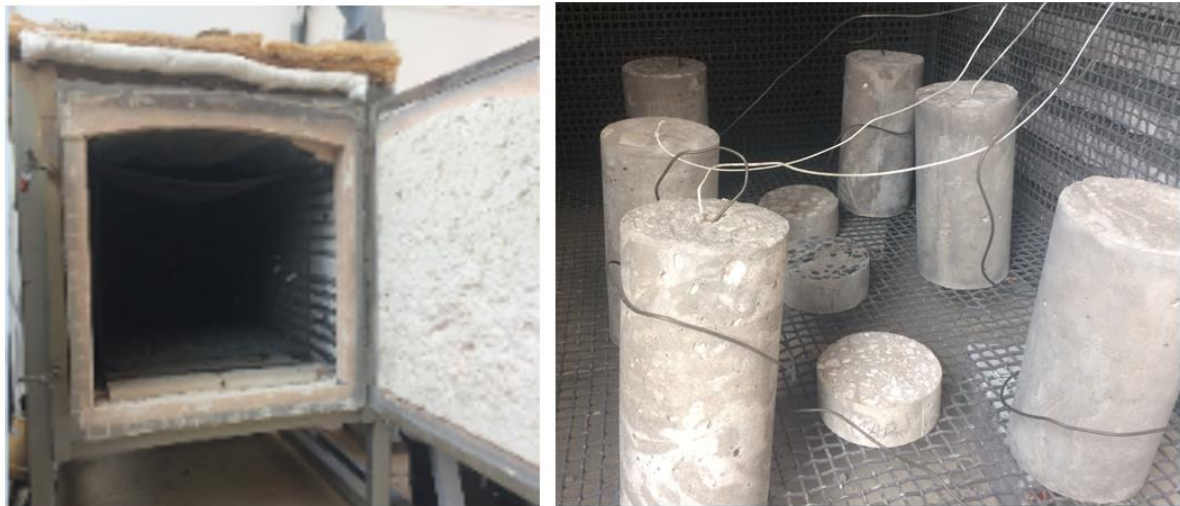
Figure 1: Left: electric arc furnace for specimens heating; right: specimens instrumented with inner thermocouples.
