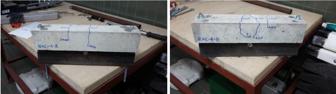
Figure 5: Position and cracks of samples NAC_NC_2 and RAC_NC_2
