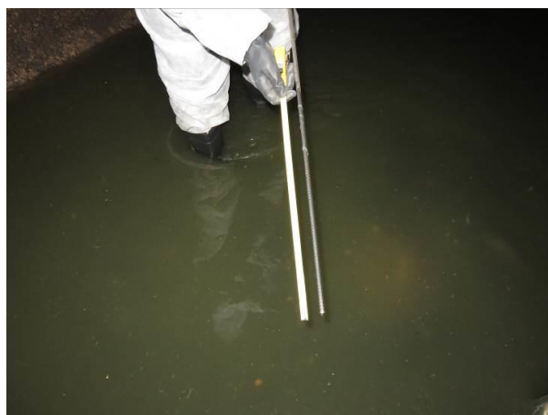
Figure 5: Sludge depth measurement
