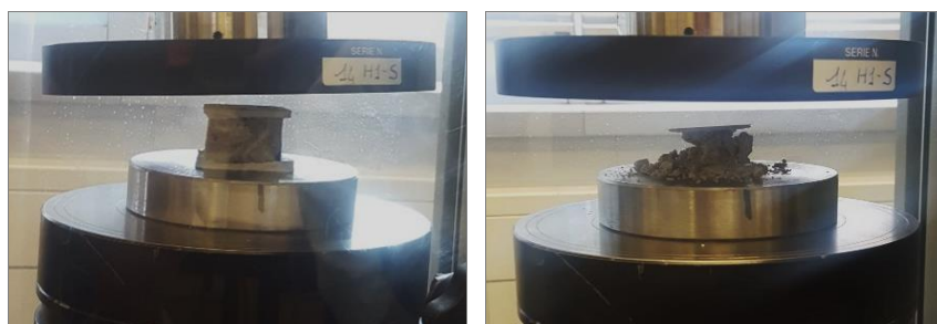
Figure 3: Compressive test of mortar specimens: before (left) and after testing (right)
