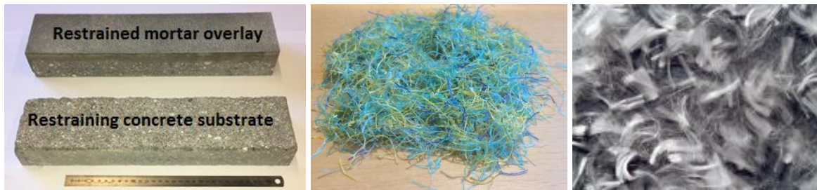
Figure 1: Geometry of substrate bases and mortar overlay; R-PE fibres; and PP fibres
