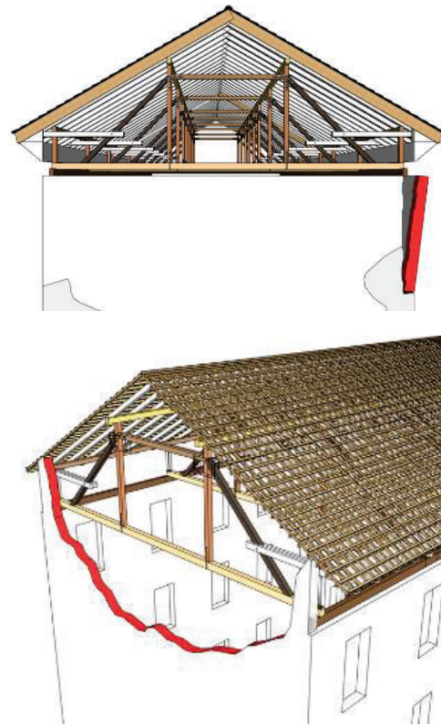
Figure 3: Typical damages to masonry walls
