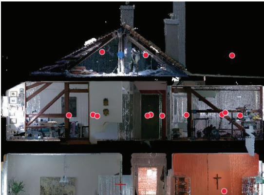
Figure 15: Point cloud of a case study building: cross section with "filming positions" (red dots)
