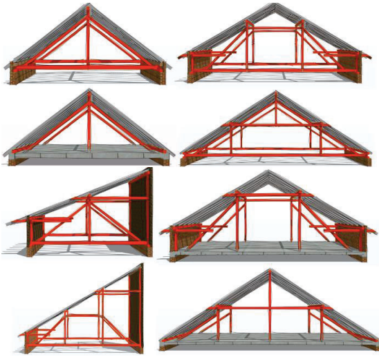
Figure 1: Typical timber roof structures in Zagreb
