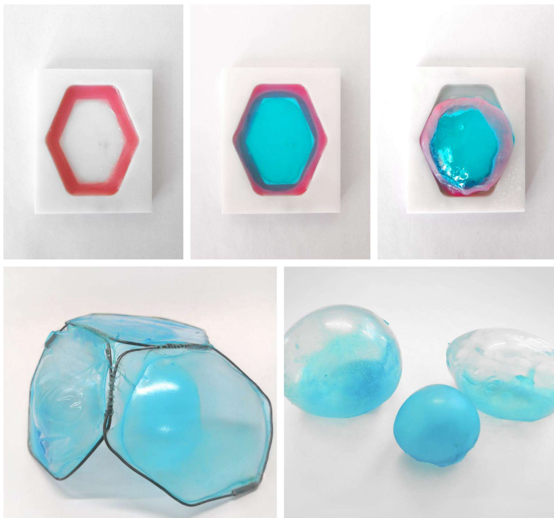
Fig. 6: top) Bonded rigid and elastic alginate (AS-04/AS-05); bottom) wire framed and free shaped air cushions (AS-05).
