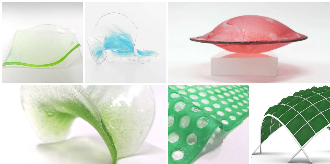
Fig. 5: top, left) Flexible foil with a controlled thickness (AS-02); top, middle) very thin membrane within a flexible wireframe, solidified material was formed into free form
