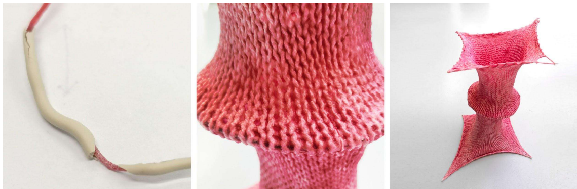
Fig. 7: left) Coating of a linear element with clay did not show promising results – due to the smooth structure of the alginate, the binding of the clay to the linear element is difficult (AS-04); middle) coating of a wool knitted structure with alginate AS-04 – wool fibres allows a good bond of the alginate with the wool structure increasing the stability of element; right) the dried part of the “Column” structure prepared for the exhibition in Pula.
