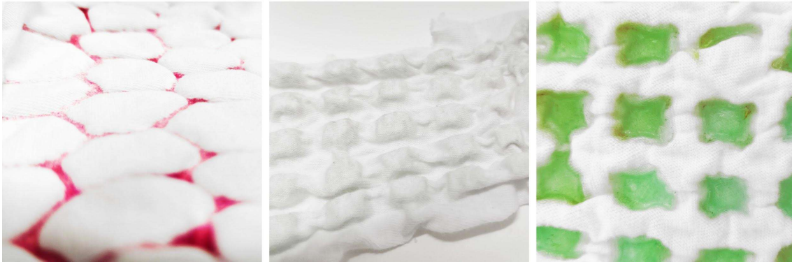
Fig. 8: left) composite of elastic fabric and AS-04 in a hexagonal matrix; middle) backside of fabric-alginate composite (AS-02) – due to rectangular alginate fields the elastic fabric is pulled together while drying; left) front side of fabric-alginate composite – alginate expands on contact with water, textile returns to its original extended form.
