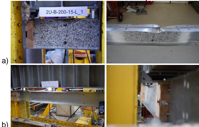
Figure 29: Deformations for 2U-B-200-1.5 a) Local, b) Interactive (Local+Global) buckling
