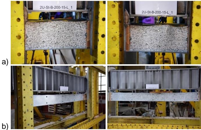
Figure 35: Deformations for 2U-St-B-200-1.5 a) Local, b) Interactive (Local+Global) buckling
