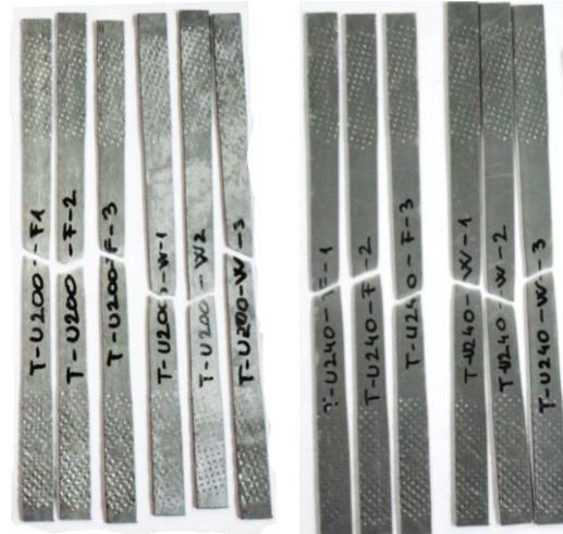
Figure 8: Tensile specimens after the test
