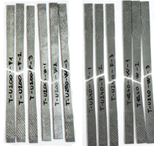
Figure 8: Tensile specimens after the test
