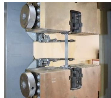
Figure 1: Steel sheet base material testing
