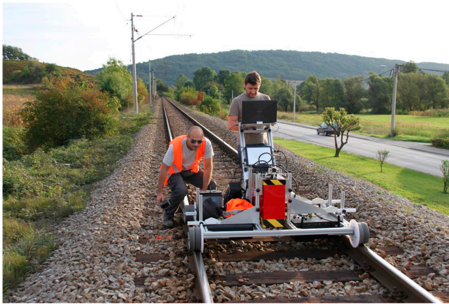
Figure 6. Conduction of GPR investigations.
