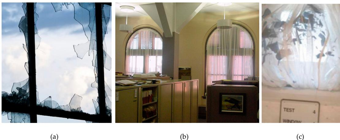
**Figure 14.** Glass windows and facades under shock: (a) example of severe damage of un-protected window and (b,c) enhanced performance in presence of textile curtain nets.
