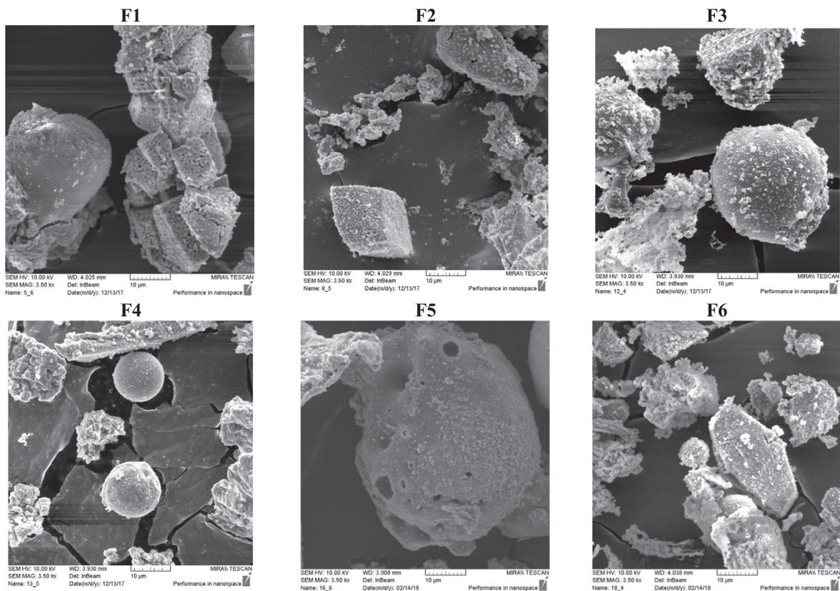
Fig. 6. Micrographs of WBAs (magnification SEM\_MAG = 3500x).
