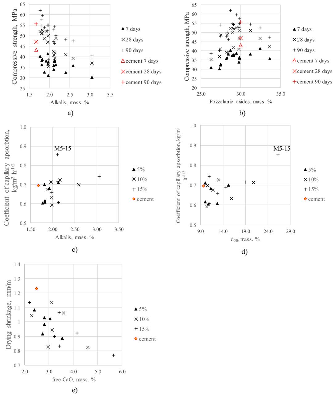
**Fig. 8.** Compressive strength of mortars at different ages compared to: a) alkali; b) pozzolanic oxides; Capillary absorption compared to: c) alkali; d) WBA size; Drying shrinkage compared to: e) free CaO.
