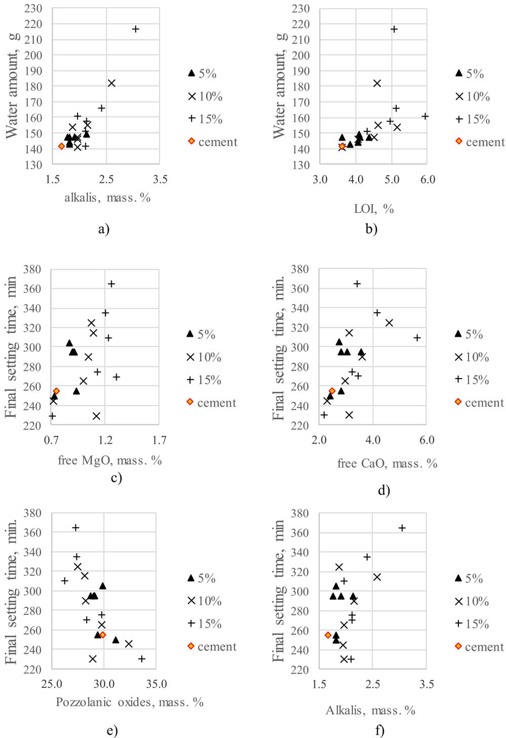
**Fig. 7.** Effect of chemical characteristics and WBA content on workability: a) alkali content, b) LOI content, and paste setting time: c) free CaO content, d) free MgO content, e) pozzolanic oxides content, f) alkali content.
