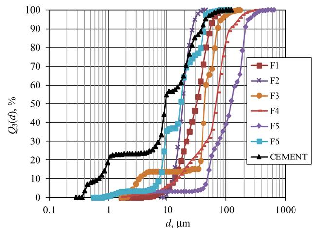
**Fig. 1.** Particle size distribution of WBA and cement.
