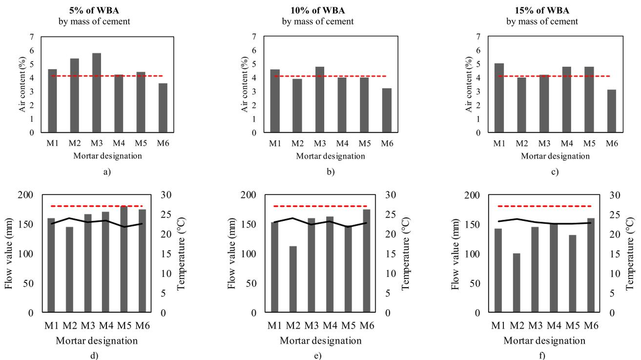
**Fig. 2.** Influence of WBA on properties of mortar based on WBAs type and content: a, b, c) Air content, d, e, f) Consistence (by flow table) and temperature (black line). \*\* red dashed lines in Figures a, b, c) represent air content of reference mix and in Figures d, e, f) flow value of reference mix.
