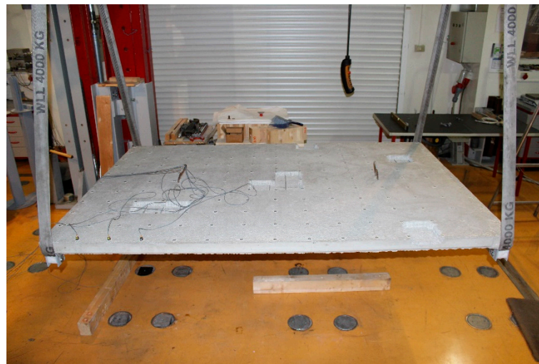
Figure 2. Suspended plate with discrete damages.
