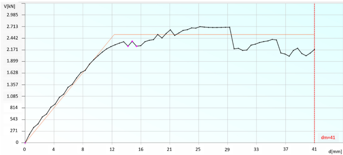
Figure 16. Capacity curve (black) and its bilinear idealization (orange) for x -direction.
