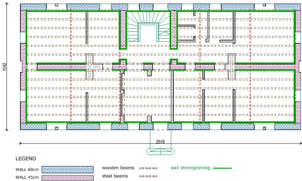
Figure 21. Proposal for reinforcement of load-bearing walls.
