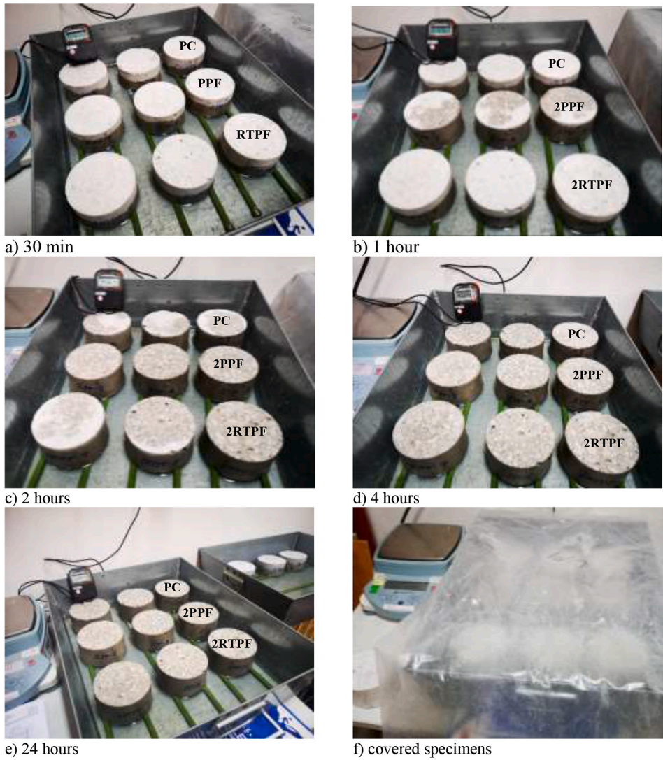
Fig. 13. Specimens heated to 500 °C for capillary absorption test at different time frames of testing.
