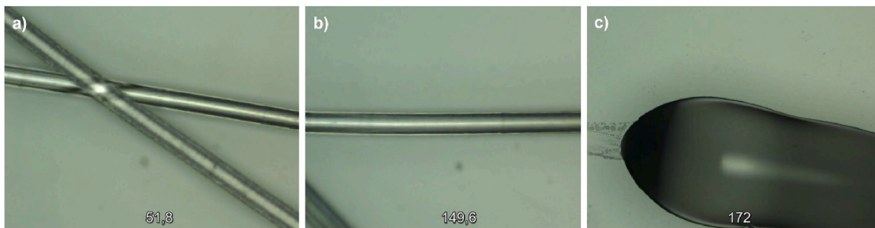
Fig. 7. a) Stable PPF (image taken at 51.8 °C), b) PPF starting to melt (image taken at 149.6 °C), and c) melted PPF increasing in volume (image taken at 172.6 °C).
