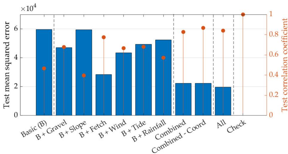
**Figure 4.** Performance statistics for tested ANNs on the test data sets according to equation 3—bar chart of mean squared errors (lower is better) on the left y-axis; stem chart of correlation coefficients (higher is better) on the right y-axis; variables included in each group can be found in Table 1; Combined group comprises Basic + Gravel + Fetch + Wind + Tide; training set, test set, and overall (training and test set) performance statistics are presented in Table A1, Appendix A.
