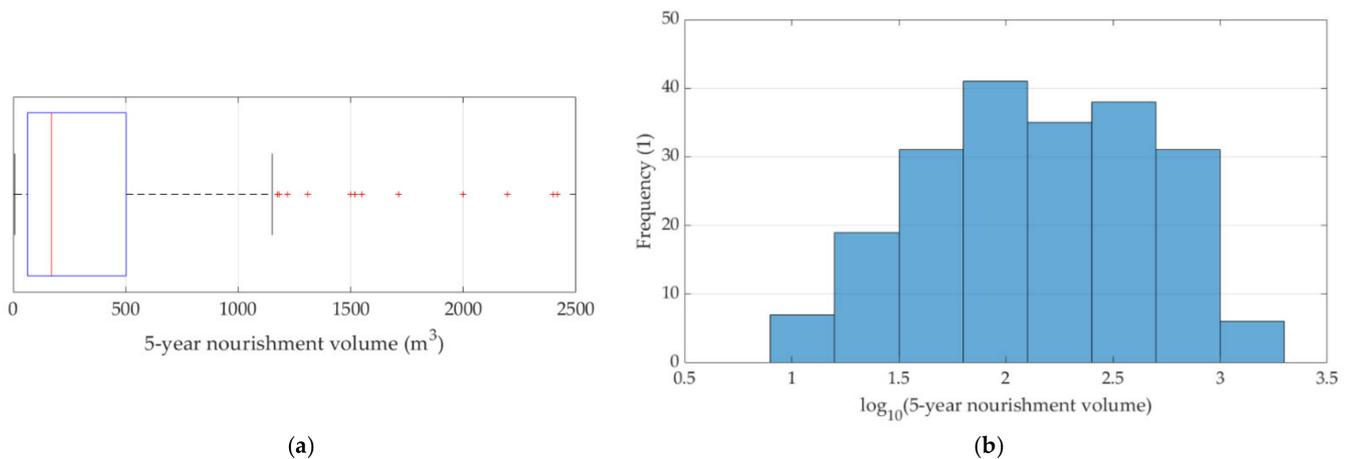
**Figure 1.** Distribution of 5-year gravel nourishment volumes that have been reported by counties in the survey: (a) box plot with specified outliers; (b) log transformed 5-year nourishment volumes correspond to a normal distribution.
