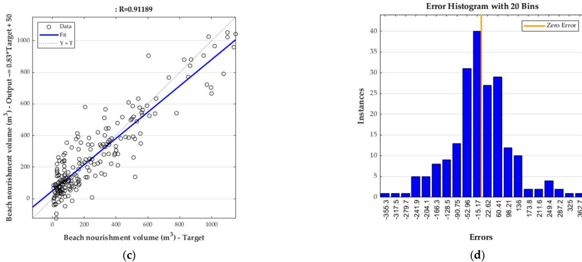
**Figure 2.** Correlation and scatter plot for the target (observed) and output (predicted using ANN) data: (a) training set; (b) test set; (c) overall (training and test set); (d) error histogram for the overall data set (training and test set) in (c).
