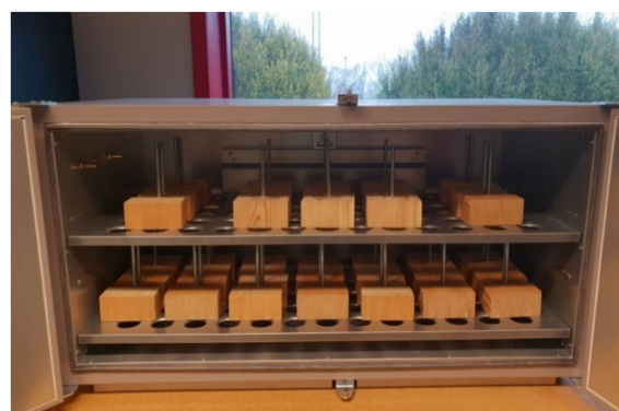
Figure 2. Preparation of specimens under controlled atmosphere.
