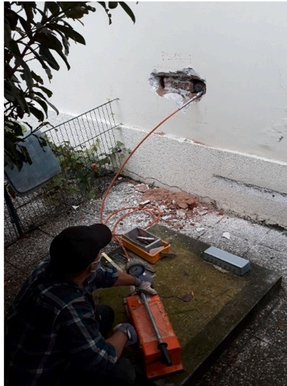
Fig. 8. Shear strength test of masonry [12].
