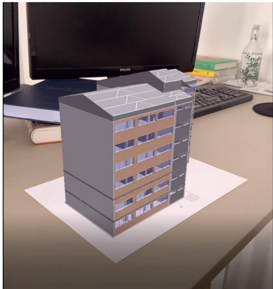
Figure 16. Scaled-down BIM model in augmented reality.
