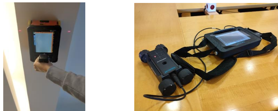
Figure 11. GPR and Profometer used for measurements.
