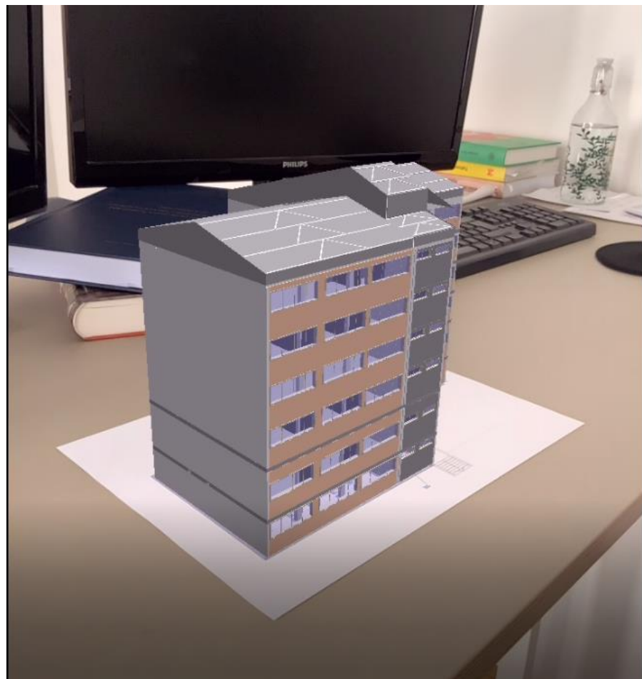
Figure 16. Scaled-down BIM model in augmented reality.
