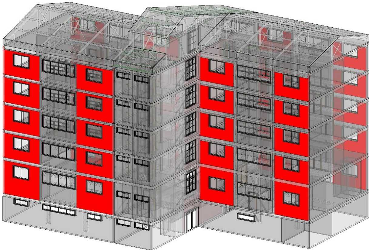
Figure 22. Additional RC perimeter walls.
