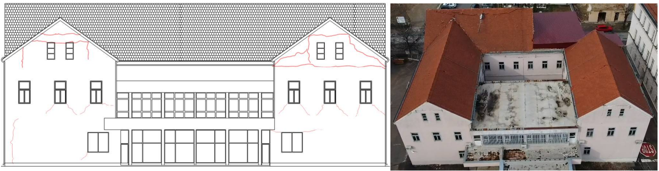
Figure 12. Northeastern façade plan with marked damage.
