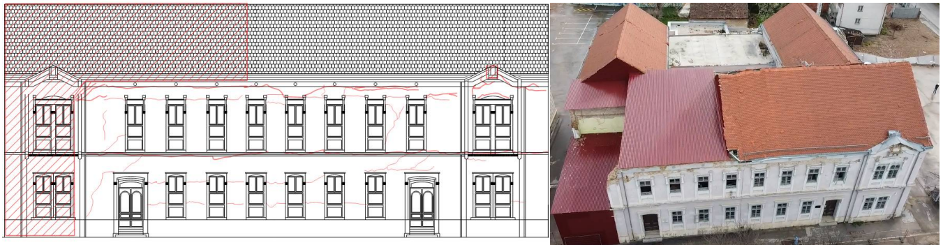
Figure 9. Southwestern façade plan with marked damage.
