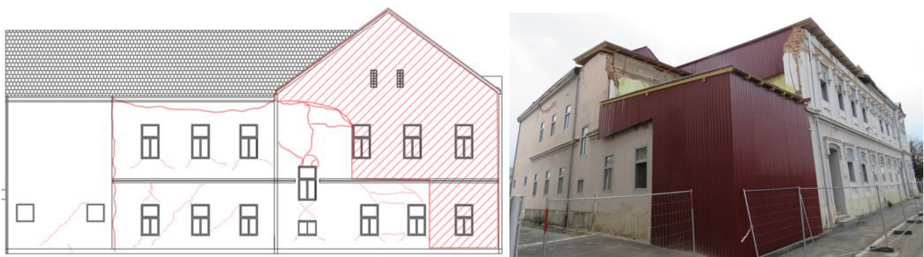
Figure 11. Northwestern façade plan with marked damage.
