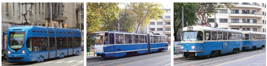
Figure 6. Types of the tram vehicles that were passing the measuring points during the field measurement: a) TMK2200, b) KT4, c) T4 (Haladin et al., 2021)
