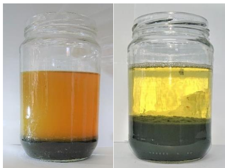
Figure 4. Observed distinction in color and quantity of flocs (after 60 min of settling): EC process operated before US (left) and US operated before EC (right).
