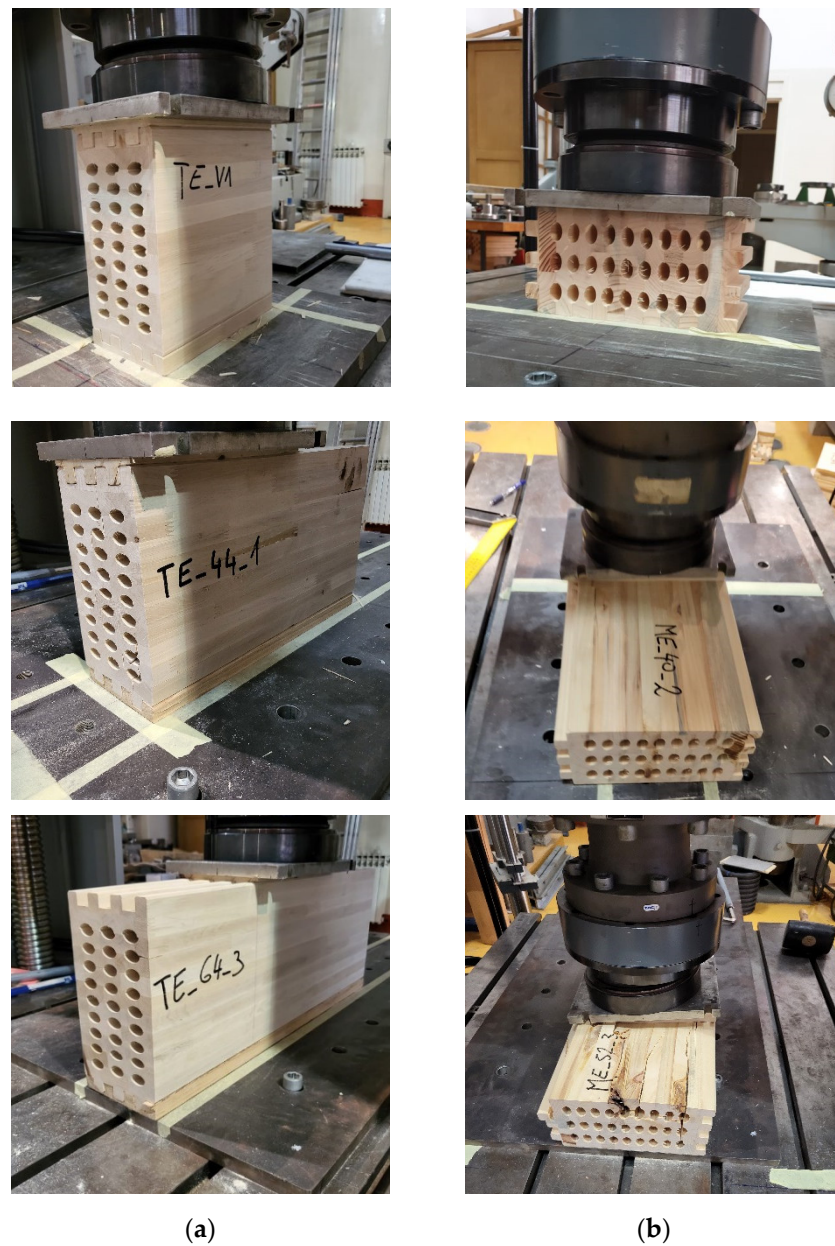
Figure 7. Loading of specimens: (a) in strong-axis direction; (b) in weak-axis direction.
