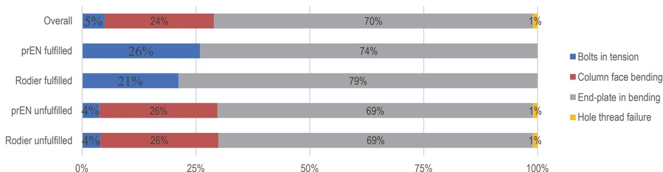
**Figure 10** Governing failure mode distributions
