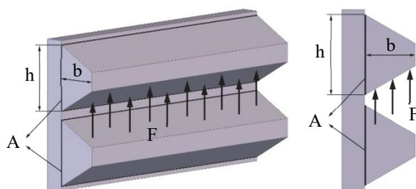
Figure 8 Force on the contact area between threads
