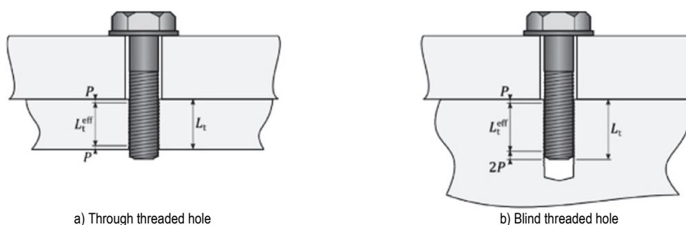
Figure 3 Bolts in threaded holes connection types [7]
