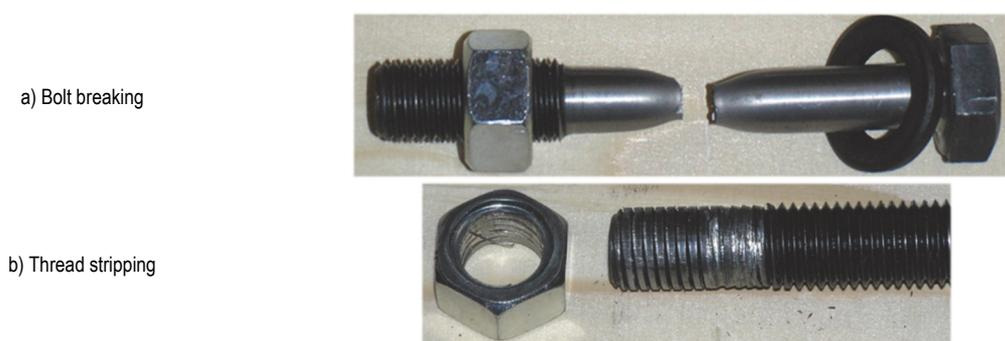
Figure 4 Bolt failure [21]
