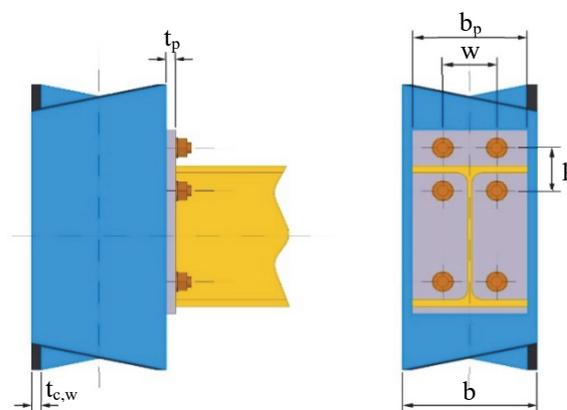
Figure 9 Analysed beam-to-column joint with an extended end-plate
