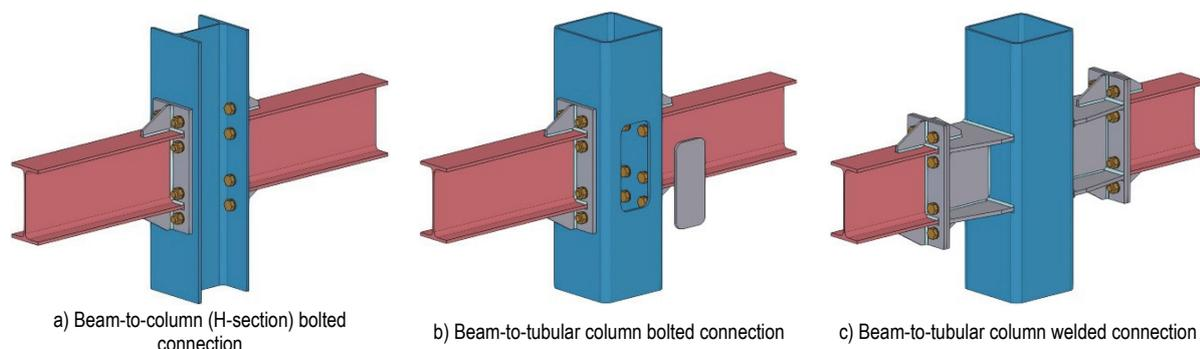
Figure 1 Beam-to-column joints
